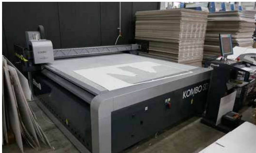
At the end of 2017 Ellerhold-Wismar bought an Elitron Kombo SD to enable prototyping staff to test their designs without interrupting production.
