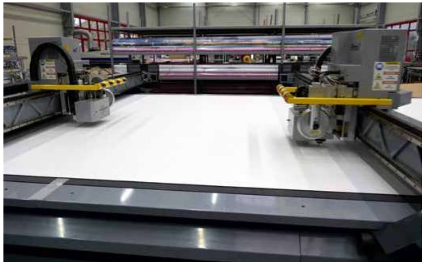
Equipped with two cutting heads, the Kombo TAV achieves a cutting speed of up to 102 m/minute.
