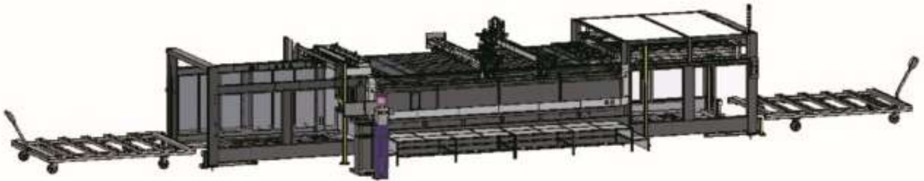
The newest Kombo K1 TAV installation: loading, cutting & creasing, unloading.
